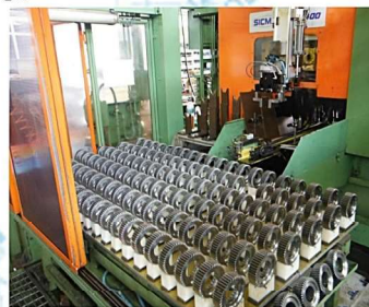
Shaving Machine robotized under 10 axes controlled
